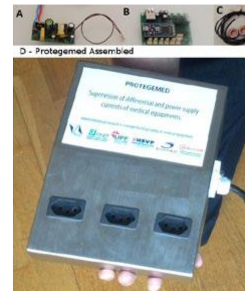
Figure 2: Protegemed Installation Kit - A: Power supply (100/240Vac to 7.5Vdc); B: Microcontroller board; C: electric current sensors (3 pairs); D: electrical outlet metal box, with Protegemed kit inside (A, B, C).
